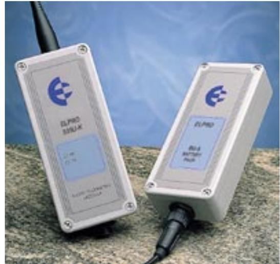
The 505U-K can be powered from a 6 - 30 VDC supply. It can also be powered from one or more ELPRO BU-5 battery packs without any other power source. Each battery pack can power the 505U-K for over a year, depending on input signal configuration. The 505U-K unit provides an internal alarm on low supply voltage - this alarm can be transmitted by radio.
