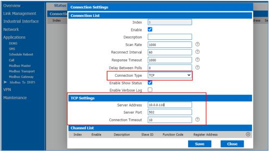
2. Go to **Applications/Modbus To DNP3/Modbus Master/Channel List**, specify the Modbus Master connection settings and the DNP3 data type:
