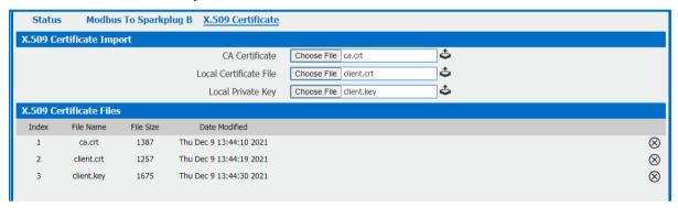
Once the certificates and key are available upload each file one at a time. For each file click Choose File, navigate to the folder that contains the files and then click the button to store in the 641M. If the file is suitable the unit will respond with Operation successful.
