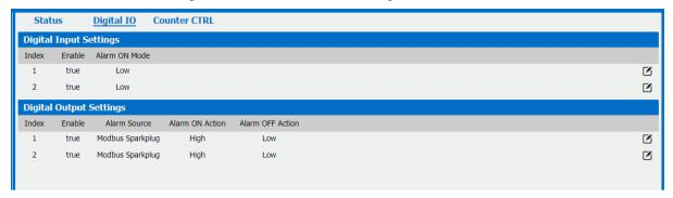
For inputs click the icon 2 and enable the digital input to allow its use.
